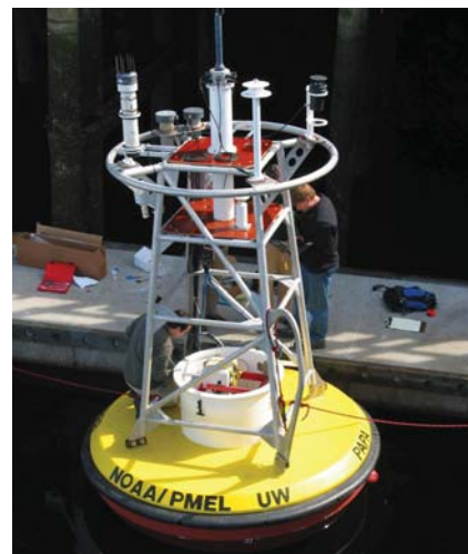
The first buoy to monitor ocean acidification, a result of carbon dioxide absorbed by the ocean, has been launched in the Gulf of Alaska, and is a new tool for researchers to examine how ocean circulation and ecosystems interact to determine how much CO 2 the North Pacific Ocean absorbs each year. Credit: NOAA
