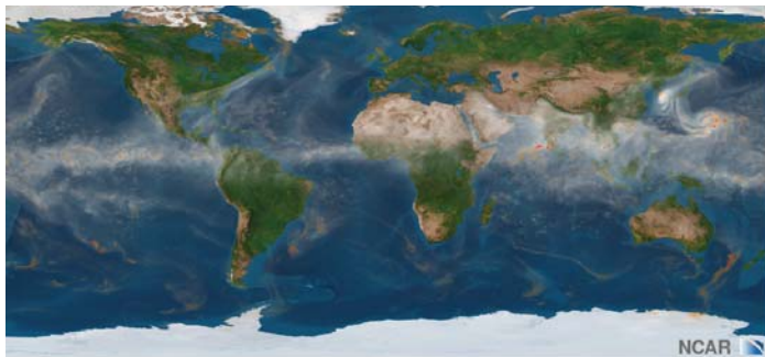
The Community Climate System Model (CCSM) simulates global cloud cover (shown in white) and precipitation (in orange). Composed of four separate models simultaneously simulating Earth's atmosphere, ocean, land surface, and sea ice, and one central coupler component, the CCSM allows researchers to conduct fundamental research into Earth's past, present, and future climate states. Credit: © University Corporation for Atmospheric Research
