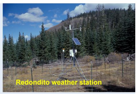
Climate monitoring: Precipitation, temperature, humidity, wind, solar radiation, soil moisture and temperature.
